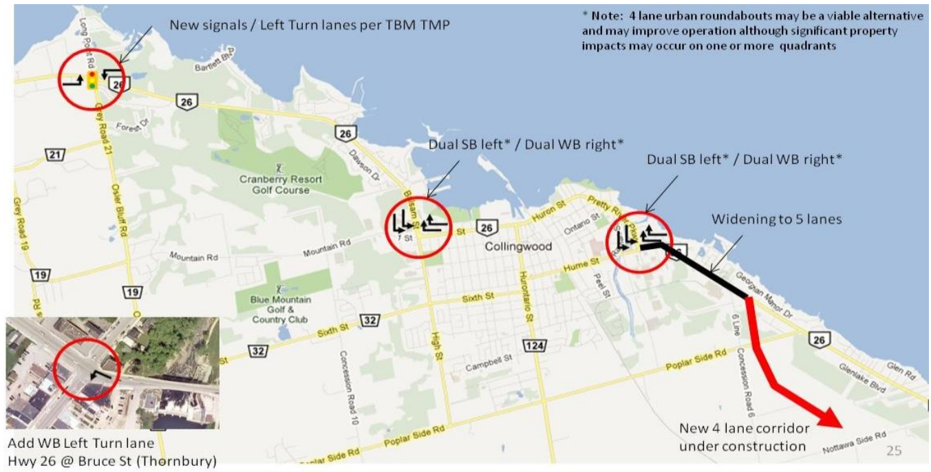
Figure 43: Tested Operational Improvements to Highway 26 Intersections
